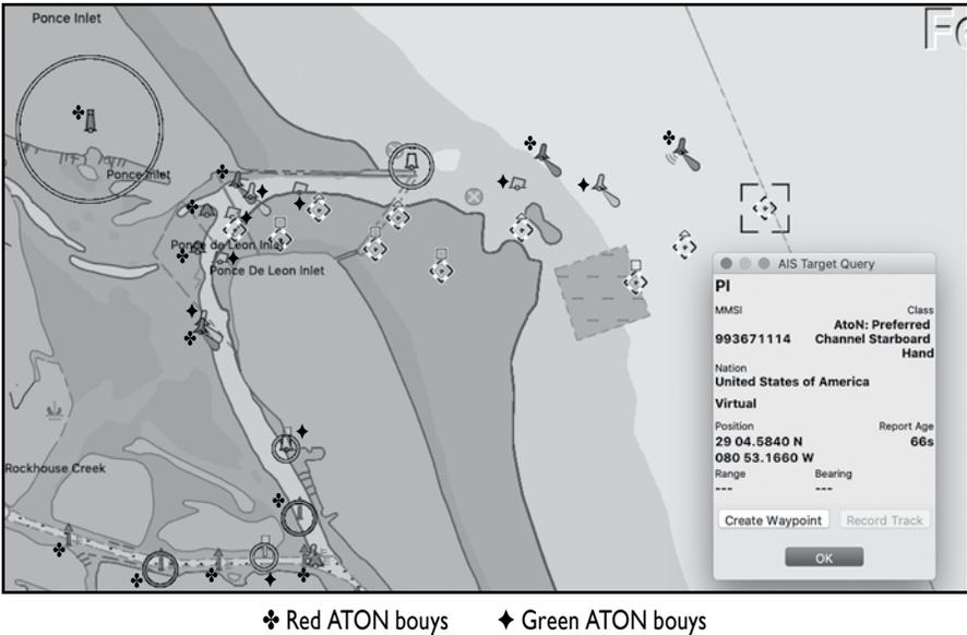
Figure 6. An AIS display of real and fake virtual ATONs is shown in Ponce De Leon Inlet, south of Daytona Beach, Florida. Source: Gary C. Kessler
