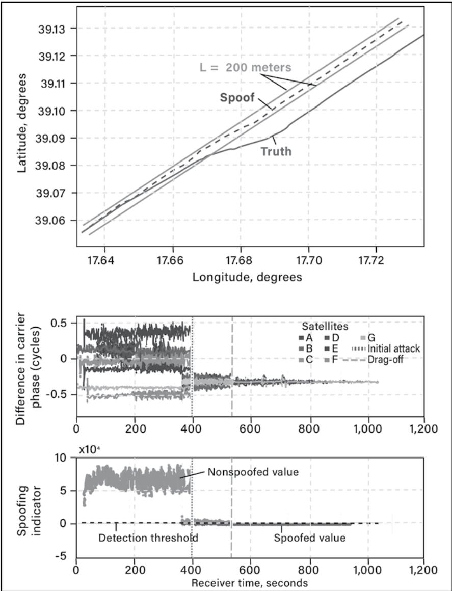
Figure 1. Anomalies appear during a GPS spoofing attack.
