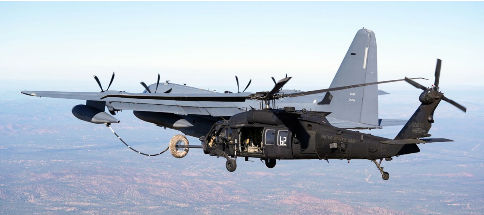
An MC-130J Air Commando II conducts helicopter air-to-air refueling with an MH-60 Black Hawk, during exercise Talisman Sabre 21 above Queensland, Australia, July 26, 2021. Source: U.S. Air Force photo by 1st Lt. Joshua Thompson
