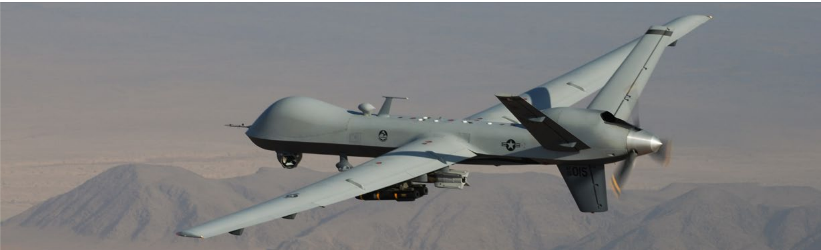
An MQ-9 Reaper, armed with GBU-12 Paveway II laser guided munitions and AGM-114 Hellfire missiles flies a combat mission over southern Afghanistan. Source: U.S. Air Force by Lt. Col. Leslie Pratt
